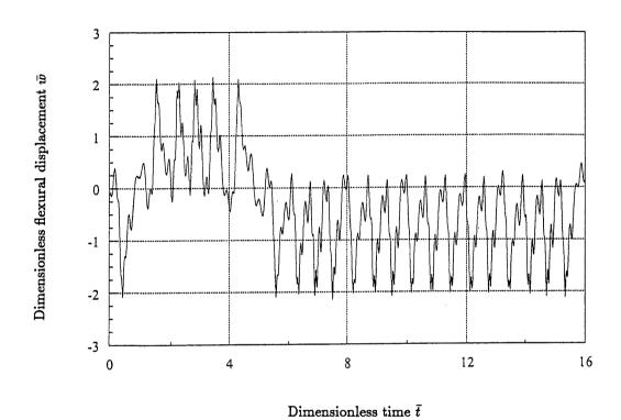
Figure 3. Plate vibration responses at  $\zeta=82.88$  ( $\zeta>\zeta_{cr,1}$  and  $\zeta>\zeta_{cr,2}$ ).
