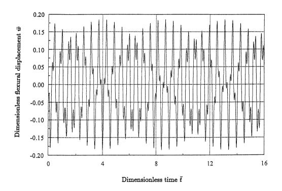
Figure 1. Plate vibration responses at  $\zeta=41.44$  ( $\zeta<\zeta_{cr,1}$  and  $\zeta<\zeta_{cr,2}$ ).
