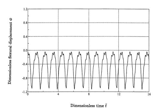
Figure 2. Plate vibration responses at  $\zeta=66.31$  ( $\zeta_{cr,1}<\zeta<\zeta_{cr,2}$ ).
